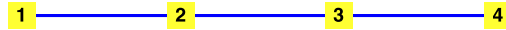
Figure 9.2. A path graph with 4 vertices has exactly 4!/2 = 12 isomorphic graphs obtained by rearranging the order in which the vertices are connected.
